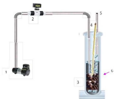
Figure 1. Schematic layout of the photoreactor used for the photocatalytic phenol degradation. 1: Air compressor; 2: Mass flow controller; 3: Phenol, water, and catalyst mixture; 4: Thermometer; 5: Air outlet; 6: Solar radiation exposure.
