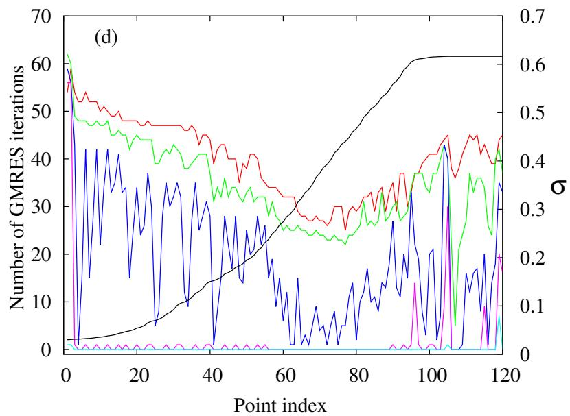
Relative distance between Newton iterates and number of GMRES iterations for the pitchfork and one of the Neimark-Sacker curves.
