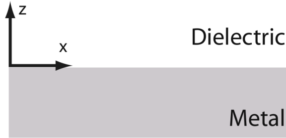
Fig. 4 Geometry of the surface plasmon-polariton propagation at an interface between a dielectric and a metal.
