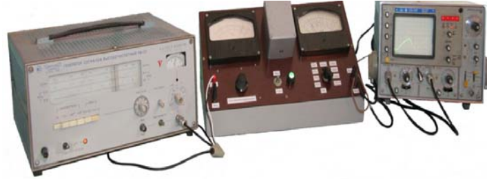
Figure 7. Installation for research of the photoconductivity relaxation.
