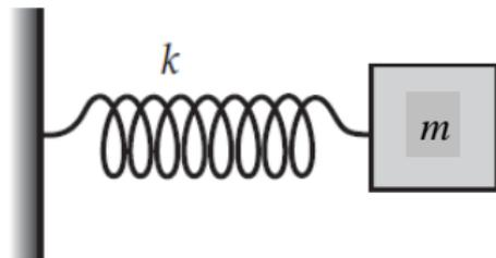
$$\begin{aligned} -kx &= F, \\ \Rightarrow -kx &= m\ddot{x}, \\ \therefore \ddot{x} + \omega_0^2 x &= 0, \end{aligned}$$
