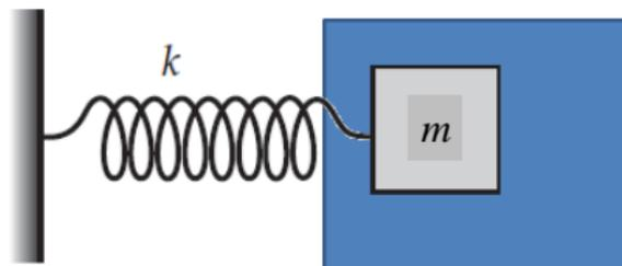
$$\begin{aligned} -kx - b\dot{x} &= F \quad \forall b > 0, \\ \Rightarrow -kx - b\dot{x} &= m\ddot{x}, \\ \therefore \ddot{x} + 2\beta\dot{x} + \omega_0^2 x &= 0, \end{aligned}$$
