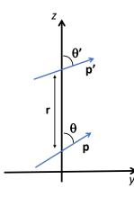
Calculate the potential energy  $U_p = -\mathbf{p}' \cdot \mathbf{E}^p$  that feels the dipole  $\mathbf{p}'$  under the influence of the electric field  $\mathbf{E}^p$  generated by the dipole  $\mathbf{p}$ , as well as the torque  $\boldsymbol{\tau}^{p'} = \mathbf{p}' \times \mathbf{E}^p$ exerted by  $\mathbf{p}$  on  $\mathbf{p}'$ , and the torque  $\boldsymbol{\tau}^p = \mathbf{p} \times \mathbf{E}^{p'}$  exerted by  $\mathbf{p}'$  on  $\mathbf{p}$ .
