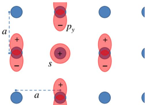
$$\begin{aligned} E_{13}(s/p_y) &= V_{sp\sigma} \left( e^{ik_y a} - e^{-ik_y a} \right), \\ E_{13}(s/p_y) &= 2iV_{sp\sigma} \text{Sen } k_y a. \end{aligned}$$
