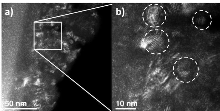
**Figure 2.** a) and b) DF-TEM micrographs of the zinc peroxide nanocrystals. The images are dominated by the contrast of Moiré fringes.
