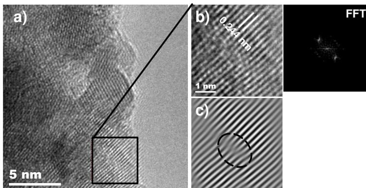
**Figure 3.** a) HR-TEM image of the as-grown ZnO<sub>2</sub> nanocrystal. b) Atomic arrangement of cubic-ZnO<sub>2</sub> nanocrystal showing the lattice fringe related to (200) planes. c) Linear dislocation exposed by filtered image technique selecting specific frequencies of FFT pattern.
