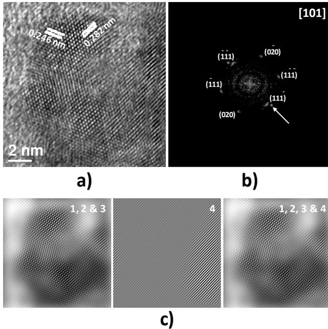
**Figure 3.** a) HR-TEM image of the as-grown ZnO<sub>2</sub> nanocrystals showing the interplanar spacing corresponding to (200) and (111) planes. b) FFT of the image shows the [101] zone axis of the nanocrystal. c) Filtered images based in the selection of the main frequencies of the FFT pattern.
