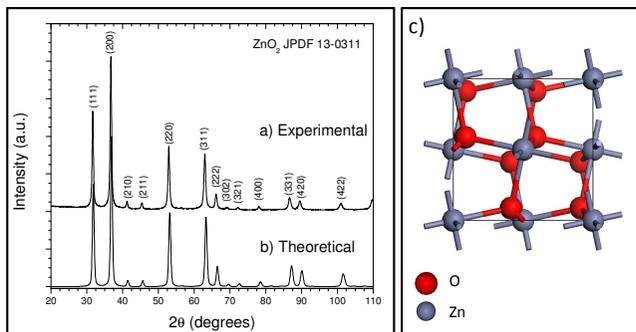
**Figure 1.** a) Experimental X-ray diffraction pattern from zinc peroxide sample. b) Theoretical X-ray diffraction pattern of cubic- $\text{ZnO}_2$  nanocrystals. c) Atomic model of the  $\text{ZnO}_2$  crystal.
