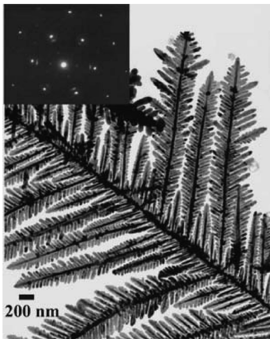
Figure 1. Typical HRTEM image of the dendritic Cu nanostructure. The sample was obtained at a potential of -1.0 V with an electrolysis time of 600 s in a 10-mL aqueous solution containing \text{CuCl}_2 (0.1 M) and \text{Na}_2\text{SO}_4 (0.1 M).
