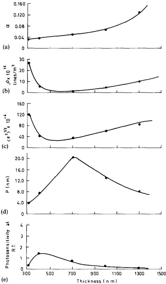
Fig. 2. (a) Stacking fault probability, (b) dislocation density, (c) microstrain, (d) particle size and (e) photosensitivity vs. film thickness.
