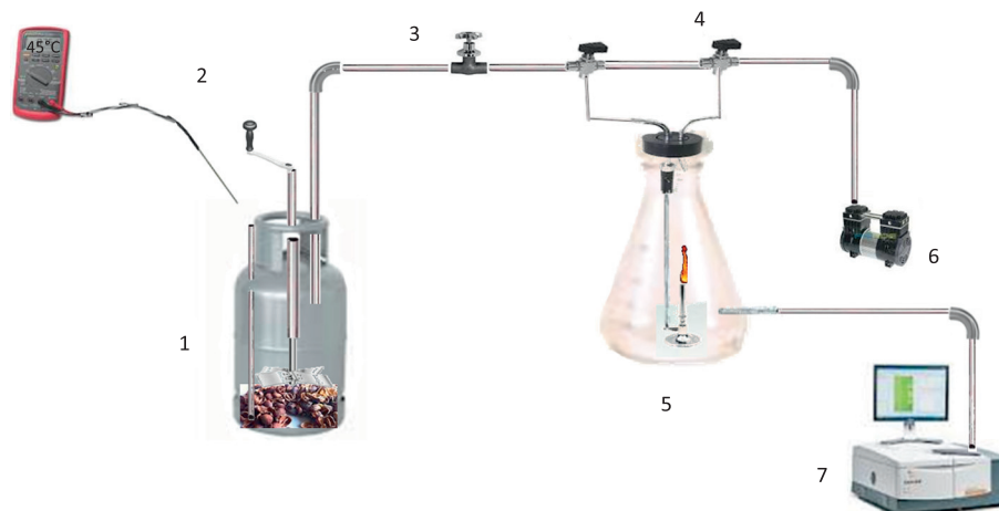
Fig. 2. Schematic layout of the biogas combustion equipment. (1) Digester; (2) thermometer; (3) biogas flow valve; (4) air flow valve; (5) biogas combustor; (6) gas compressor; (7) FTIR spectrometer.
