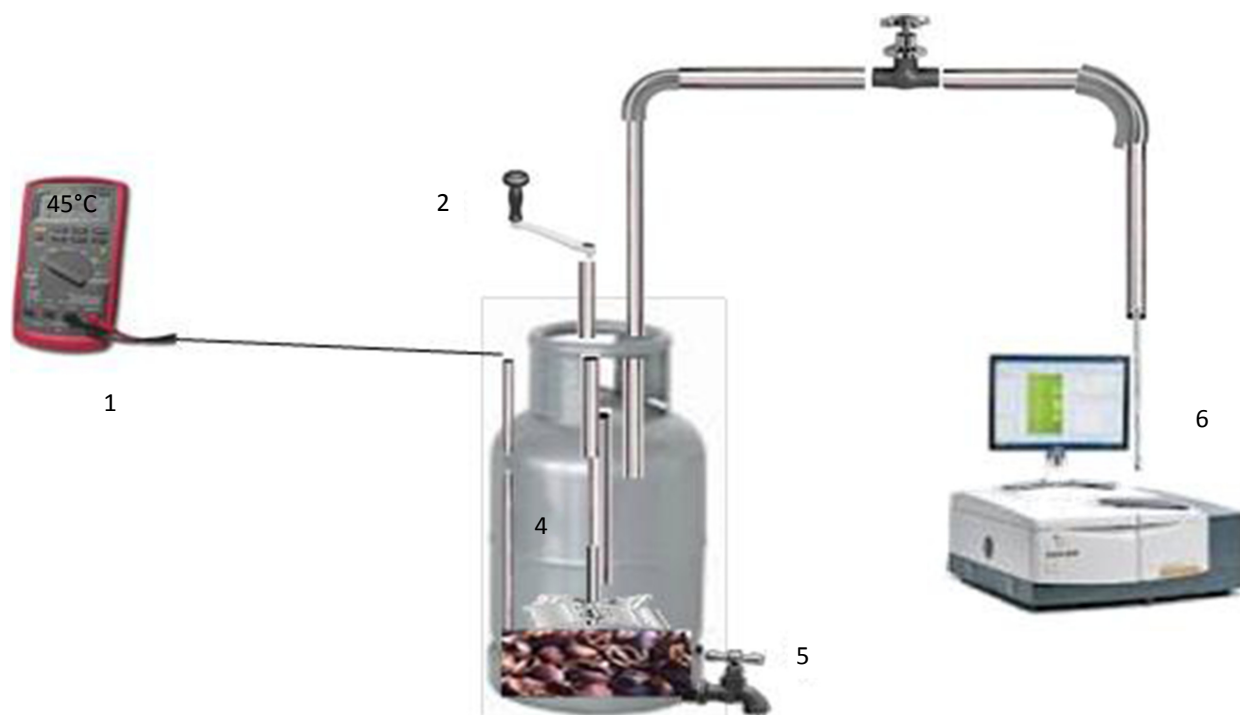
Figure 2. Schematic illustration of the used codigestion setup (1): thermocouple; (2): mixing crank handle; (3): activated carbon; (4): digestion reactor; (5): sampling valve for pH measurement; (6): FTIR spectrometer.
