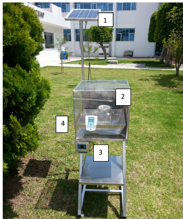
Fig. 1. Solar reactor used for biodiesel production: (1) photovoltaic cell, (2) heating chamber, (3) solar energy driven magnetic stirrer, and (4) solar power meter.
