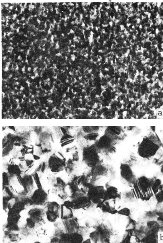
Figure 6. TEM photographs (with magnification \times 66000 ) of \text{Cd}_{0.8}\text{Zn}_{0.2}\text{Te} thin films deposited at (a) 300 K and (b) 575 K.
