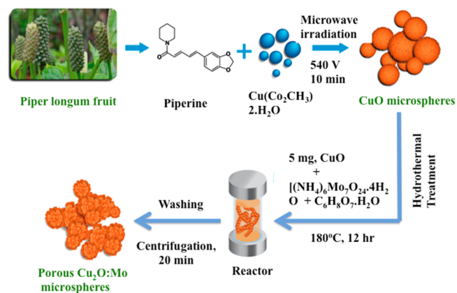
Figure 1. Schematic illustration of the two-step synthesis process utilized for fabricating porous Cu 2 O:Mo microspheres.
