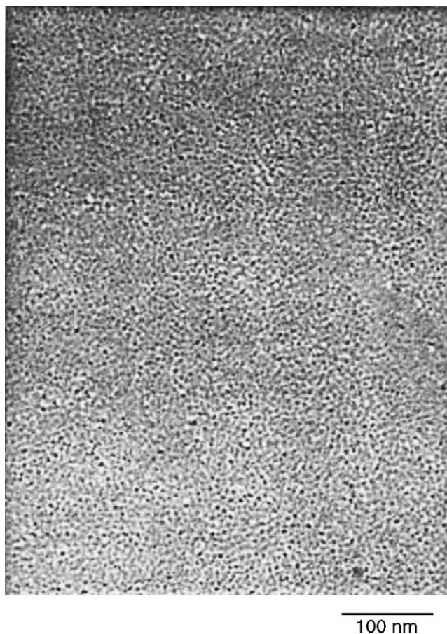
Fig. 2. TEM photograph of as-deposited Si/ZnO film prepared with 12 Si targets.
